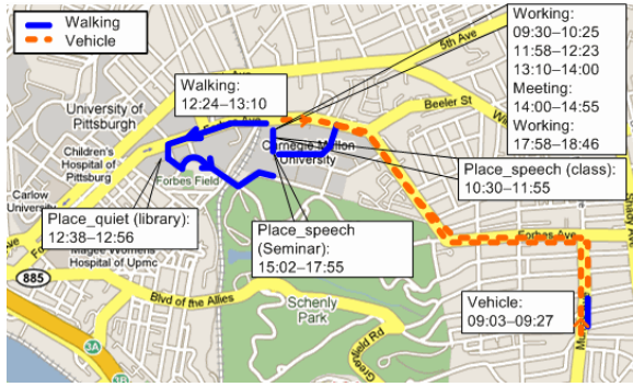
Figure 7: Recognized daily activities of a sample CMU user. The figure shows the time, user location as well as background sound condition detected by EEMSS.
