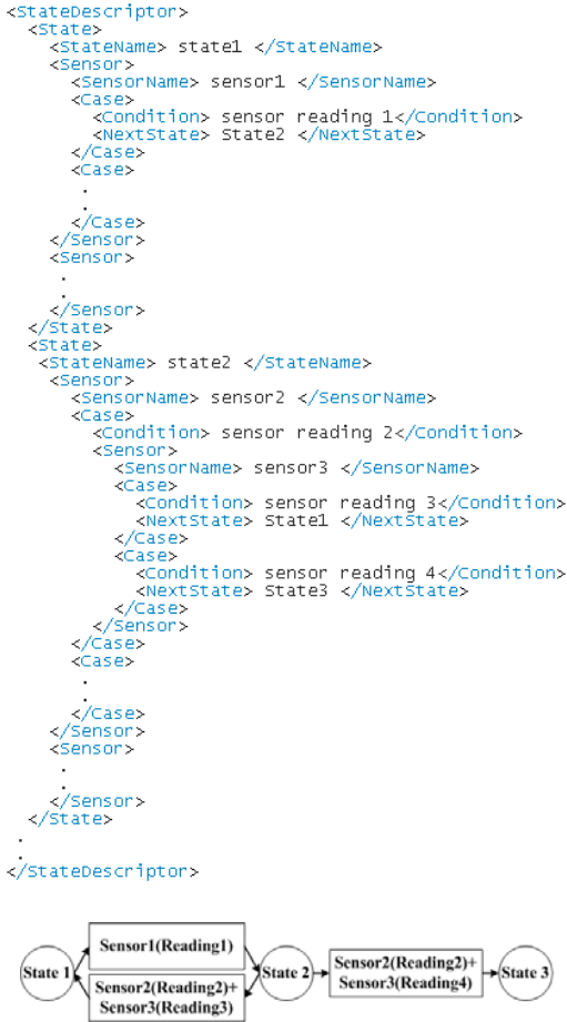
Figure 1: The format of XML based state descriptor and its implication of state transition.
